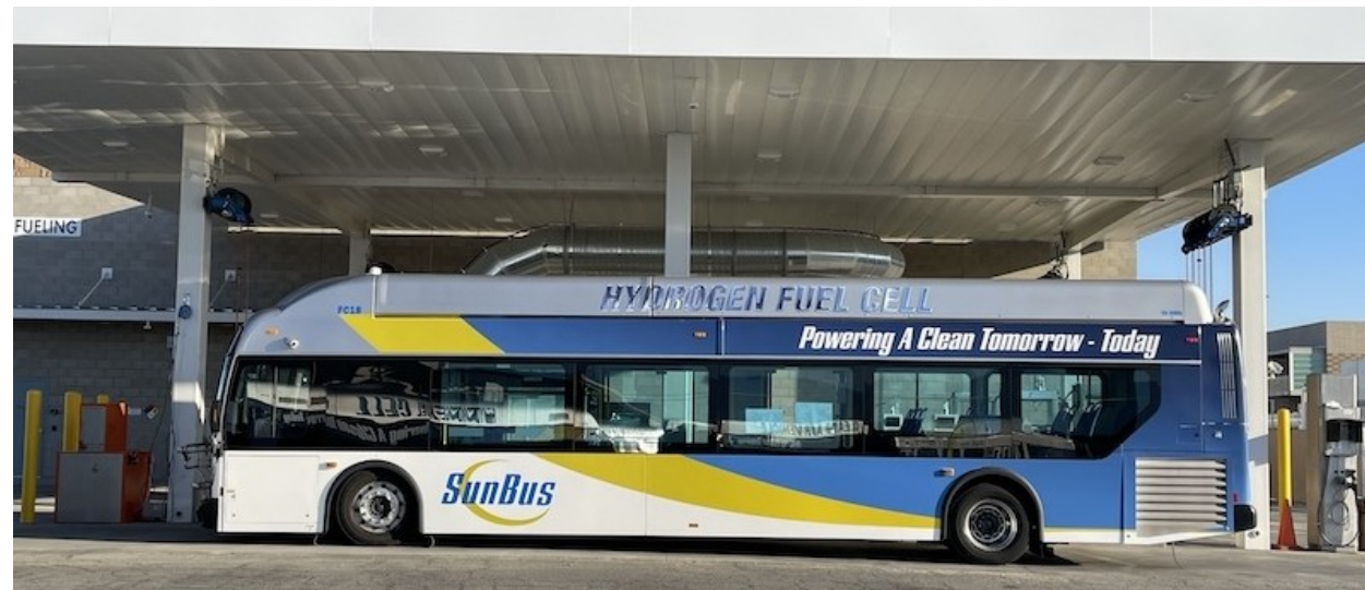
A SunLine Transit hydrogen bus at a hydrogen fueling station (source: sunline.org)
