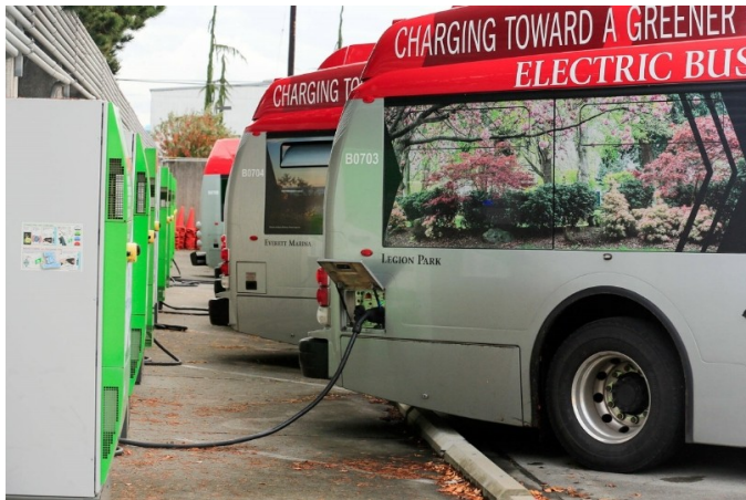
Plug-in Charging for a BEB (source: heraldnet.com)
