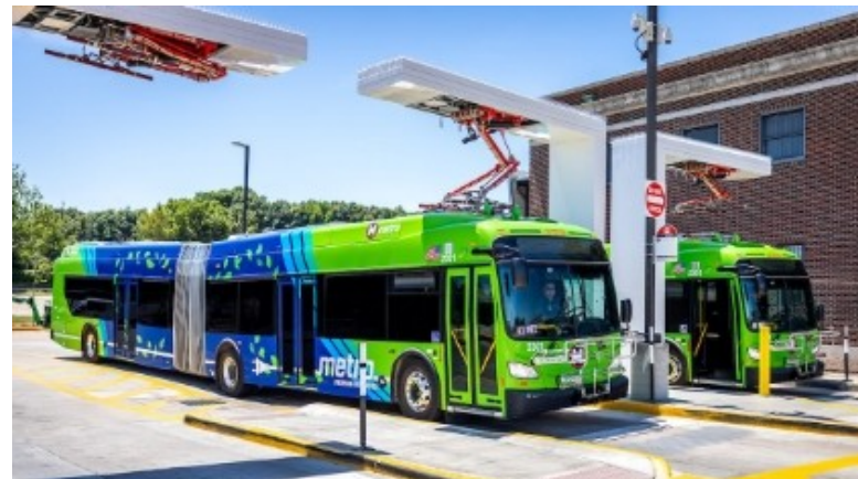
Overhead Pantograph Charging (source: metrostlouis.org)
