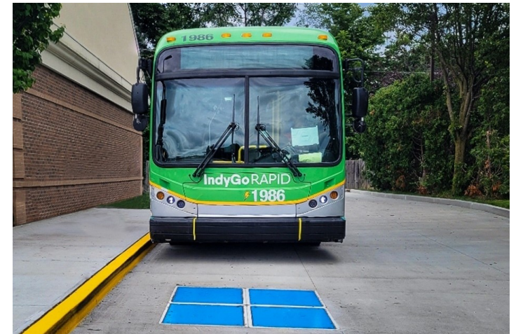
An IndyGo Rapid transit bus approaches a wireless charging pad (source: chargedevs.com)
